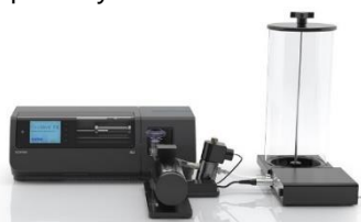
Figure 1 - The flexiVent FX equipped with the FEV Extension
