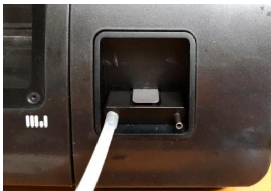
Figure 9. Testing the inspiratory cartridge+ inspiratory side of the adapter
