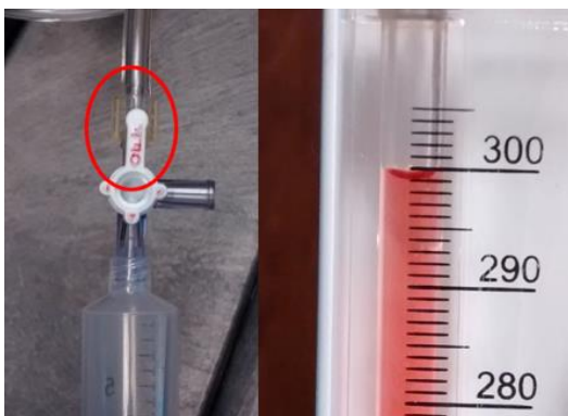
Figure 4. how to close the manometer
