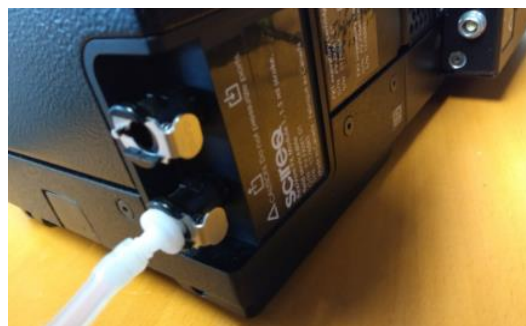
Figure 8. Testing the air exhaust port
