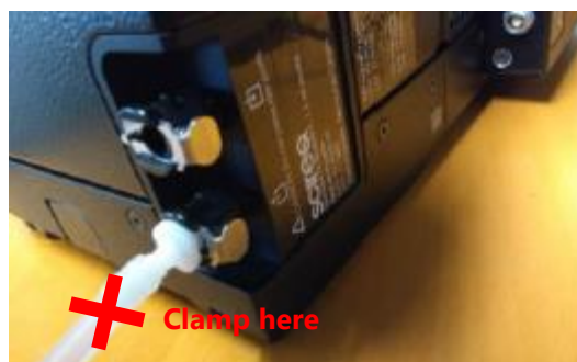
Figure 12. Testing expiratory + adapter +Y-tubing
