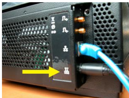
Figure 2. The back of the FX, power port indicated
