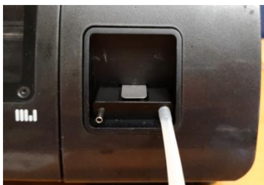
Figure 10. Testing the Expiratory cartridge and expiratory side of the adapter
