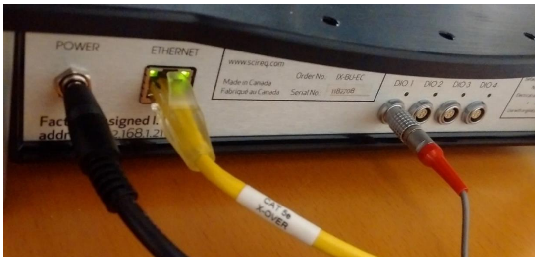
Figure 2-7: Power (BLACK), Ethernet (BLUE or YELLOW), & Trigger (GREY/RED) cables on the back of the inExpose
