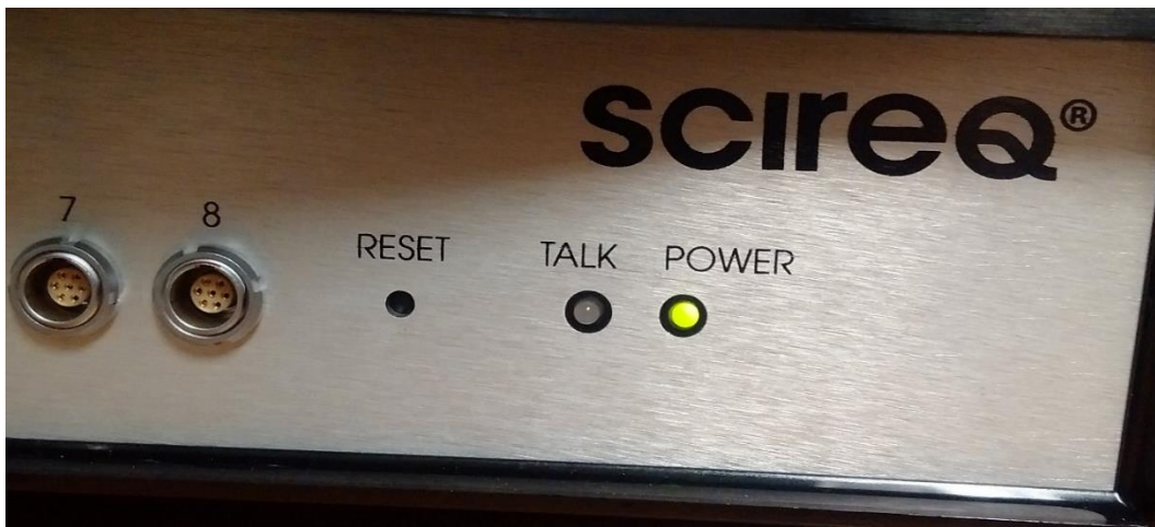
Figure 2-9: Reset button & LED on the front of the inExpose when the system is available for connection or connected to the software
