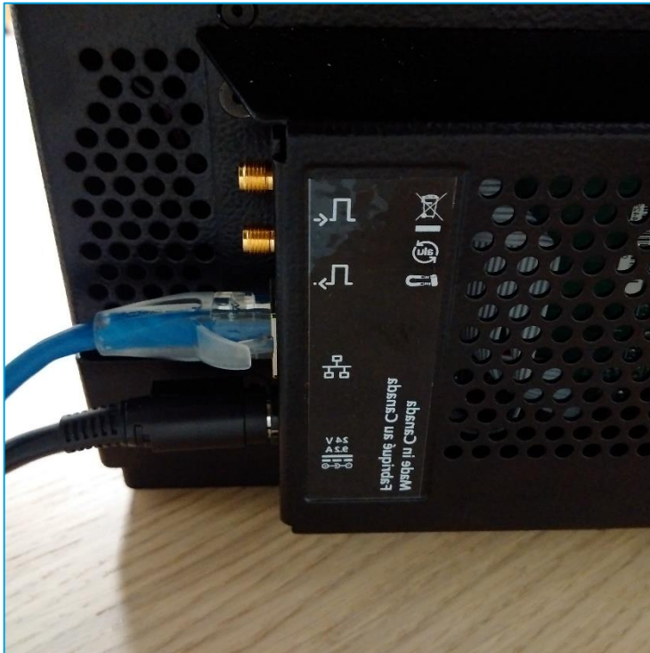
Figure 2-8: Power (BLACK) and Ethernet (BLUE or YELLOW) cables on the back of the flexiVent
