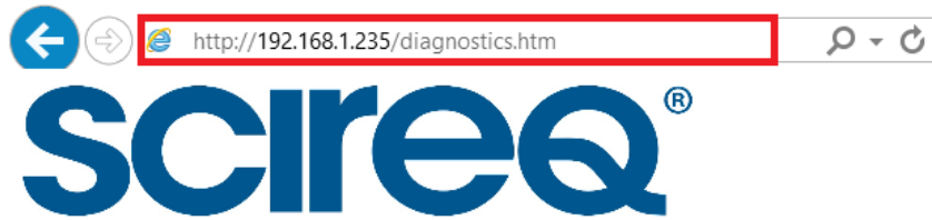
Figure 2. Type Diagnostics address into web browser for firmware version 8.0 or higher
