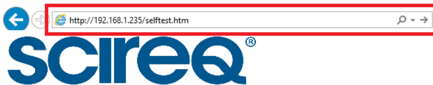
Figure 3. Type SelfTest address into web browser for firmware version 7.6
