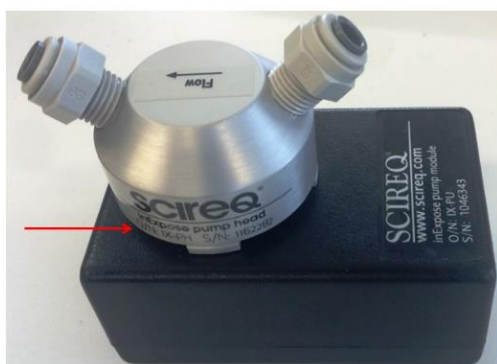
Figure 1. The Diaphragm pump with pump head firmly attached (red arrow)
