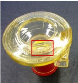
Figure 8. The standard aeroneb head with mesh portion indicated
