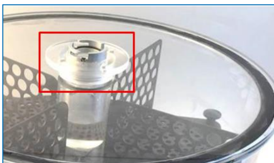
Figure 5. WBC lid with portion used to tighten the lid indicated
