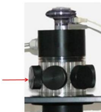
Figure 6. The nose only tower with one of the black plugs used to seal the tower indicated
