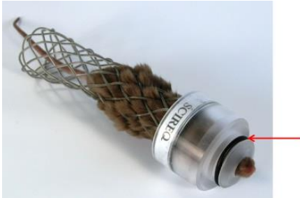
Figure 7. A softRestraint with mouse inserted snugly, o-ring of restraint highlighted
