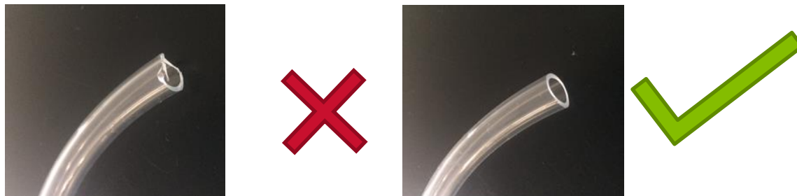
Figure 4. Tubing ends must be cut perpendicular and evenly(right), not jagged or with uneven ends (left) to assure good seal
