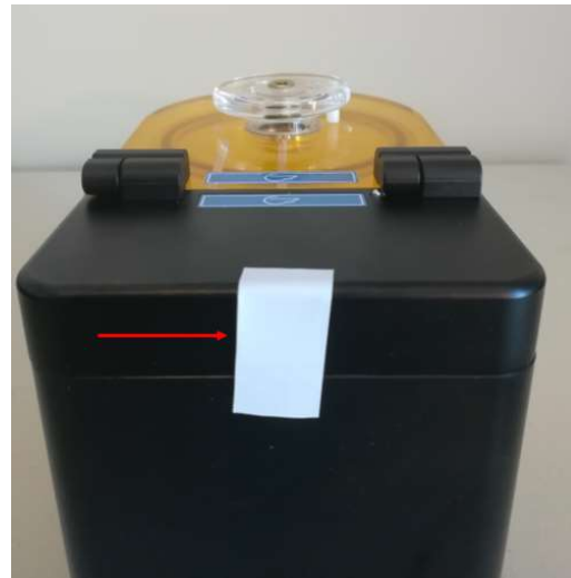
Figure 4: Tape to seal off the concentric pneumotachograph on the back of the VF
