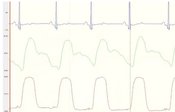
Figure 3: Real-time measurements displayed by IOX software, showing an EKG waveform (top), aortic pressure (middle), and left ventricular (LV) waveform (bottom)
